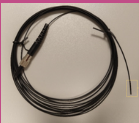
Final ORIGIN optical fibre sensor showing scintillating tip following UV excitation
