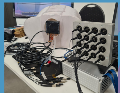
R; Demo of prostate HDR BT procedure with ORIGIN sensors placed within the target, urethra and rectum.
