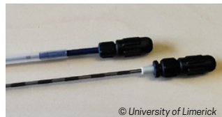
Fibre securement device to fix the optical fibre sensor within the brachytherapy needle
