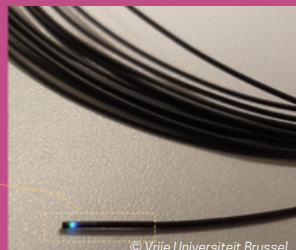
Final ORIGIN optical fibre sensor showing scintillating tip following UV excitation
