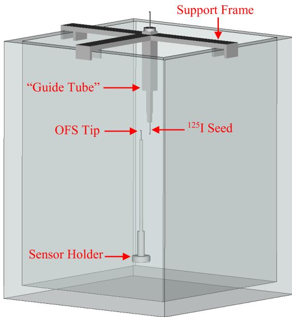
**Fig. 2.** Water phantom experimental setup employed for acquiring measurement data. The  $^{125}\text{I}$  seed (within a plastic needle) and the sensor tip (also within a plastic needle) are labeled, as are the 3-D printed components. See the Appendix for schematics, including dimensions, of 3-D printed components.
